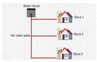
District heating properties are served from a main boiler house. These pump hot water into the radiators and cylinders in each property.
